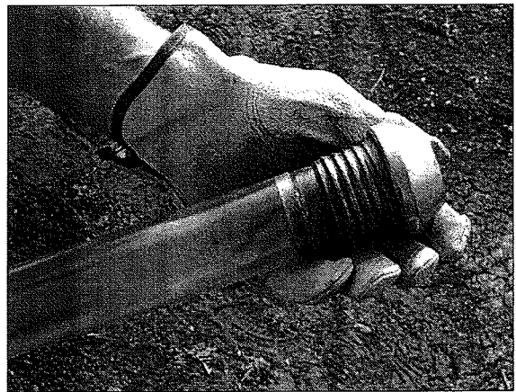
Figure 4.19. Place either end of the liner onto the extended shank cutting shoe. (This is used in place of a spacer ring or core catcher)
