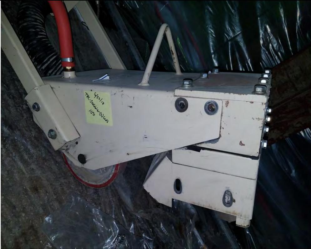
Photo 29: Side of scabbler following decontamination and wipe sampling.
