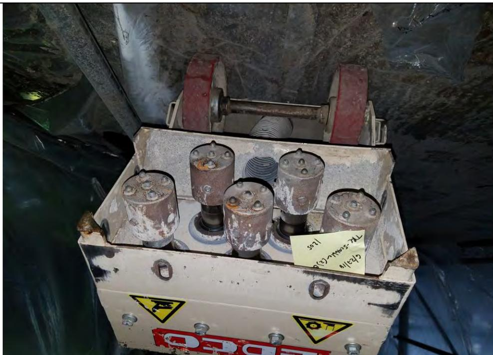
Photo 28: Underside of scabbler following decontamination and wipe sampling.
