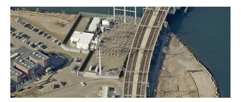
During Superstorm Sandy (October 2012), when flood waters encroached to within inches of the control room floor, again UI preemptively de-energized the substation due to the risk of equipment failure and long-term recovery issues. The purpose of the project is to build a flood protection system that will mitigate the risk of damage to the substation equipment from similar weather events in the future.
